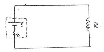
6-16. In problem 6-12 if the wires are connected as shown here, now what is the resistance AB and the current in each if  $V_{AB} = 10V$ ?
